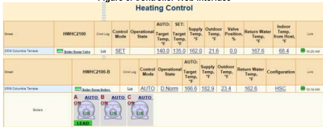
Figure 7. Mixing valve controller (top) and boiler controller (bottom) Web interface
